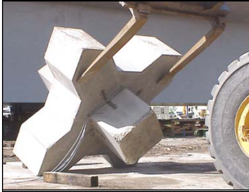
Figure 2: Photograph of Overturning – Cubical Leg test set-up.
