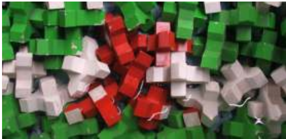
Figure 1 - cluster of broken Xbloc armour units (in red)
