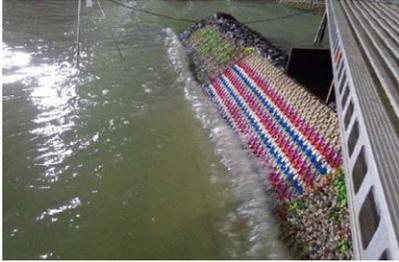
Figure 3 - Wave attack during 3D tests
