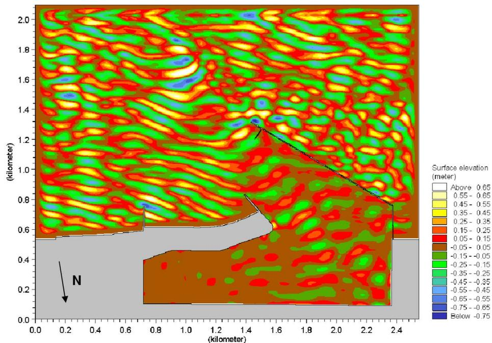
**Figure 8** Wave model, diffraction around main breakwater
