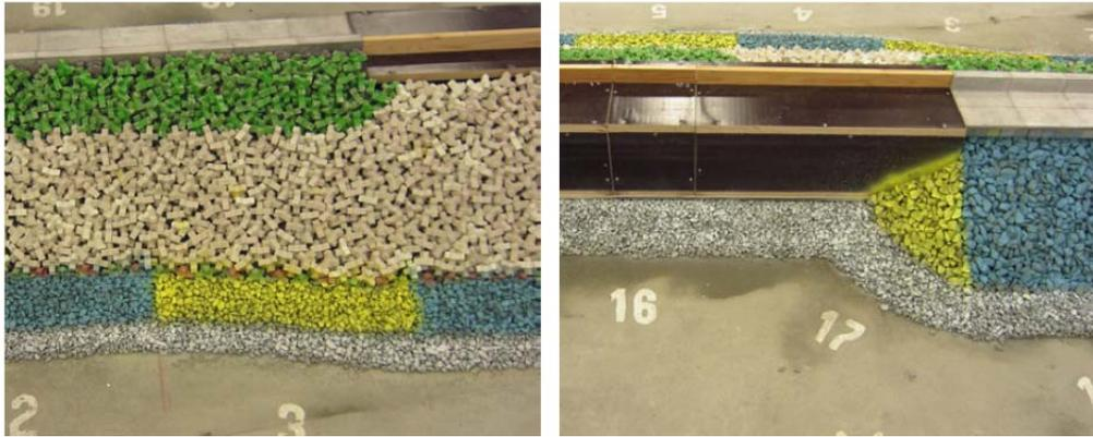
**Figure 4 Transition zone between caisson and rubble mound breakwater**
