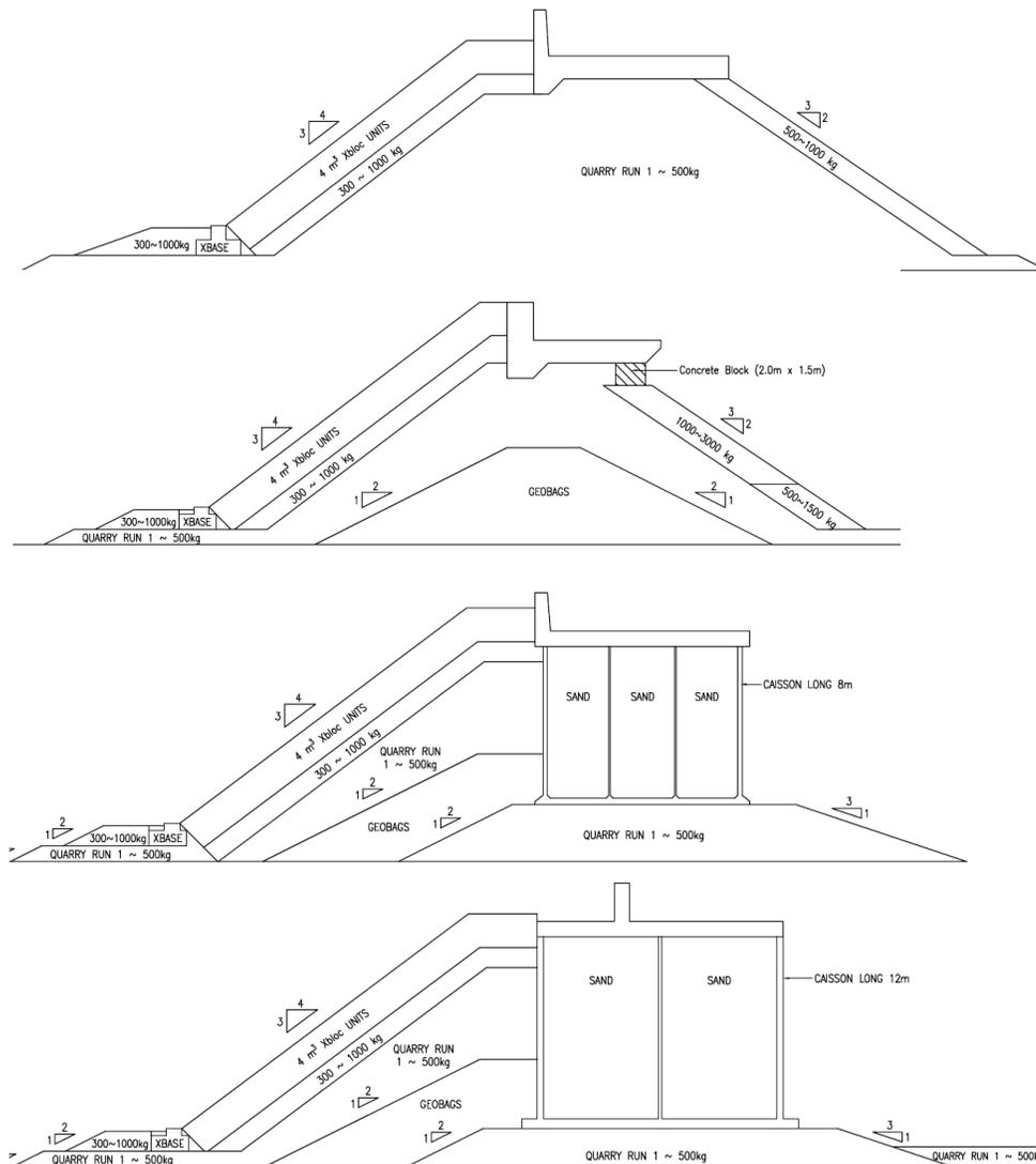
**Figure 2 Cross sections main breakwater: (a) Conventional rubble mound structure (top); (b) rubble mound structure with core from geotextile containers (2<sup>nd</sup> from top); (c) composite breakwater (2<sup>nd</sup> from bottom); (d) final layout of composite breakwater (bottom);**
