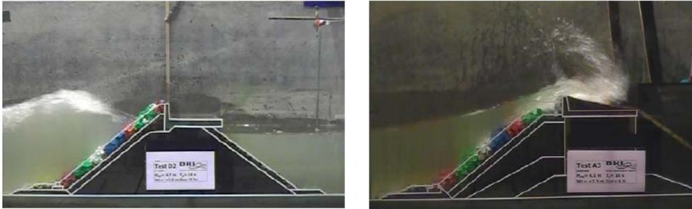
**Figure 3 Cross sections of main breakwater (2D model tests)**
