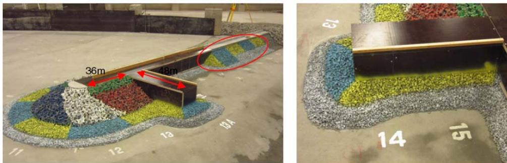
**Figure 5 Spur breakwater (altered rear side armour layer circled)**
